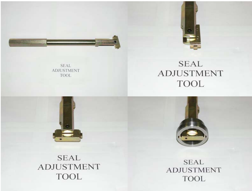
PLUG SEAL ADJUSTMENT TOOL SHOWN WITH BASE PARALLEL TO SHANK FOR INSERTION, BASE PERPENDICULAR TO SHANK, AND ENGAGED IN SEAL ADJUSTMENT NUT.
